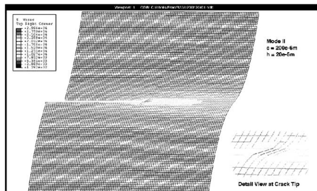
Fig. 14. Deformation of the foam subjected to Mode II loading (cell length c = 200 \mu\text{m} , strut thickness h = 20 \mu\text{m} ).
